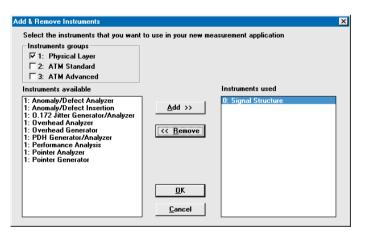
The <u>"Add & Remove</u> <u>Instruments"</u> window opens. It shows all the available instruments. A list of instruments in use is shown on the right. Those not yet in use are shown on the left.
